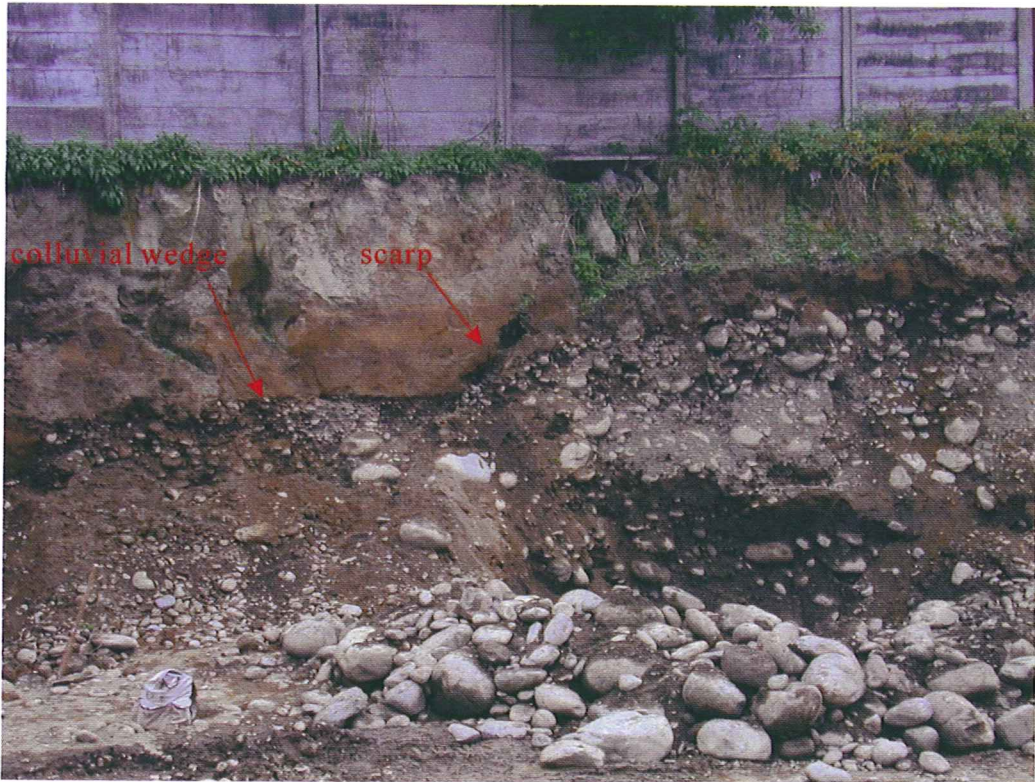
Figure 3. Top of the gravel layer formed a free surface representing an obvious fault scarp of about 1.2 m height during the paleoseismic I event. On the downthrown side of the rupture I is deposited wedge-shaped colluvial deposits. In addition, several sand and paleosol layers unconformably cover the scarp.
